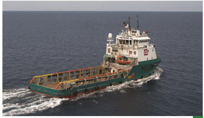
PSV is a state of the art platform supply vessel. Equipped with Diesel Electric propulsion, three main engine configuration, triple stern L-drives, two bow thrusters, and Dynamic Positioning Class II (DP II), the vessel is extremely maneuverable and capable of precise station keeping while in DP mode while also making operations extremely safe and reliable.
